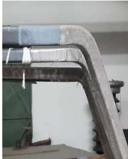
End Corona Coating section of bar
