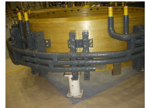
Coated Bus Bars in Support ring
