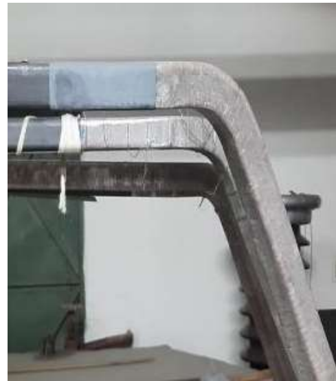
End Corona Coating section of bar
