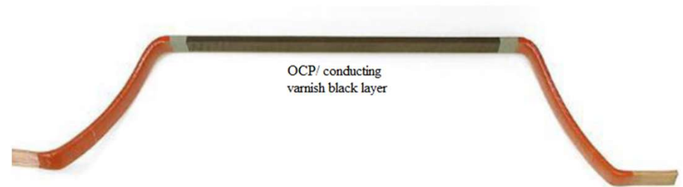
Stator bar coated with OCP Varnish
