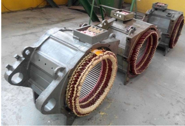
Stator after VPI
